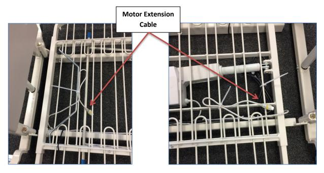
9. Plug the motor extension cable into the high low actuators. Then install the "C-Clips" that are in the bag with the user manual, these should lock in place (Step 4). Followed by, fastening the remaining cord to a washer with a tie strap provided.
