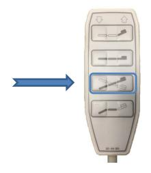
The up arrow will raise the head of the bed and lower the foot of the bed simultaneously putting the resident in the Trendelenburg position. The down arrow will raise the foot of the bed and lower the foot of the bed simultaneously putting the resident in the Reverse Trendelenburg position.
