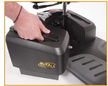
Step 2: Pull out the battery pack!
