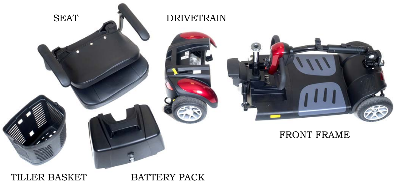
Figure 18. Buzzaround XL™ Components (Model GB147)
