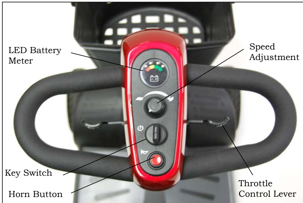
Figure 5. Buzzaround XL™ Delta Tiller Control Panel
