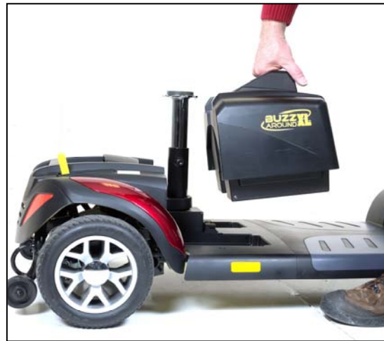
Figure 15. Removing the Battery Pack
