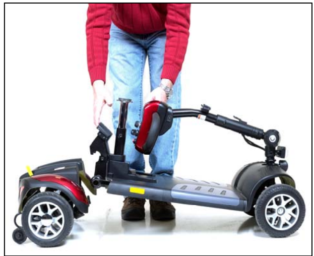
Figure 20. Connecting Frame and Drivetrain
