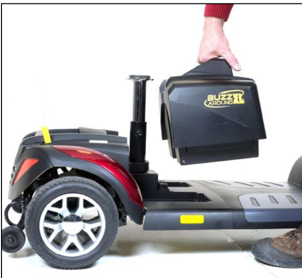
Figure 21. Battery Pack Installation
