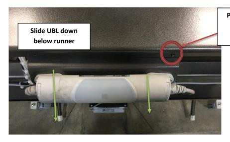
Place tab through hole for proper alignment
