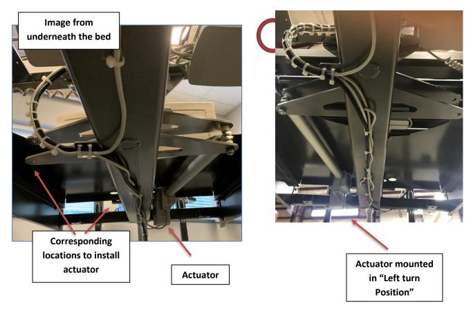
Install fasteners and spacers back in actuator. Tighten the fastener so that the bolt comes through the nylon nut but do not overtighten or the actuator will bind causing damage,
