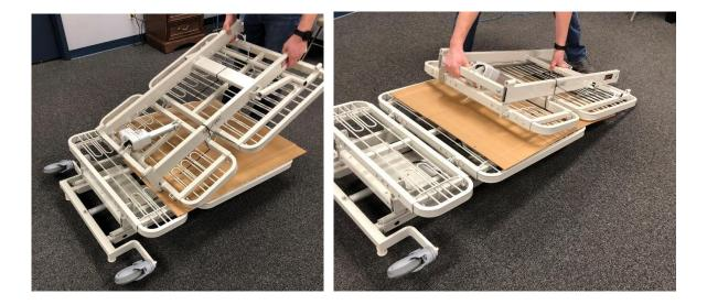
7. Unbolt the other two 7/16-14" X 4 ½" Bolts and remove the head section assembly from the head high low assembly. Remove and retain hardware for assembly process.
