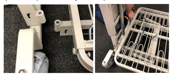
3. Turn each bolted together assembly over to orient the bed decks like below and align the welded bosses directly with each other.
