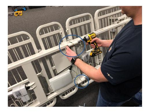
5. Use the two 7/16-14" X 1  $\frac{3}{4}$ " bolts and nuts to secure the inside frame to each assembly. Be sure to use the impact drill again to firmly secure.
