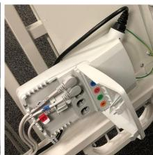
7. Plug cables 3 (Green) and 4 (Orange) into the respective locations. Route the cabling to seat into he groves of the control box and then close tightly.
