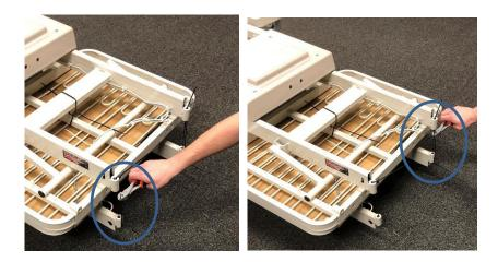
4. Near the casters are two 7/16-14" X 4 ½" zinc bolts, these need to be removed with the 5/8" socket and drill. Retain these bolts and nuts for assembly process.
