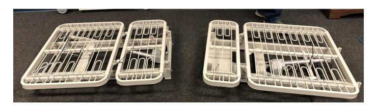
9. There are two more 7/16-14" X 1 ¾" bolts that need removed, located on the foot end deck assembly, retain hardware for assembly process.
