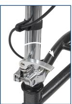
4. Insert pad post into receptacle on frame. Secure pad in place by inserting locking pin into hole. Lock pin in place by sliding retainer tab into position.
