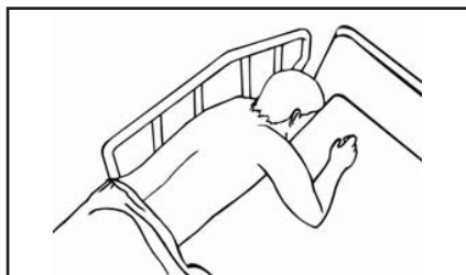
Zone 3 – Entrapment between the rail and the mattress
