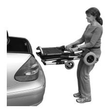
Next, grab the Cross Tube to lift the Zinger off the ground with the Battery cradle pressed against your thighs.
