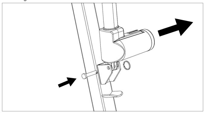
**Step 6**: Install upper end of the actuator by using the quick-release pin.
