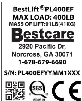
The manufacturing date can be found on the serial number label that is located at the top of the mast. The YY in the serial number is the manufacture year, and the MM is the manufacture month.
