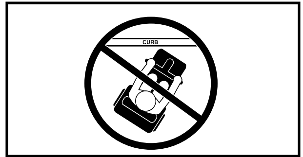
Figure 7. Incorrect Curb Approach
