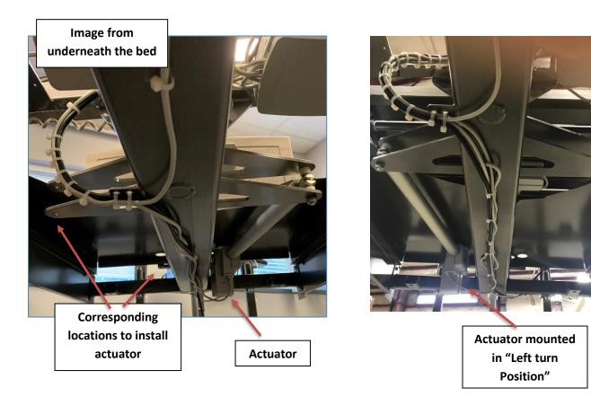
3. Install fasteners and spacers back in actuator. Tighten the fastener so that the bolt comes through the nylon nut but do not overtighten or the actuator will bind causing damage,
