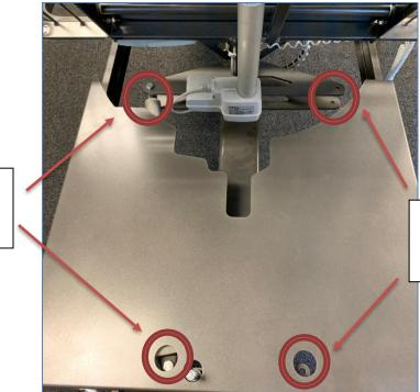
Remove bolts using 17mm wrench and socket
